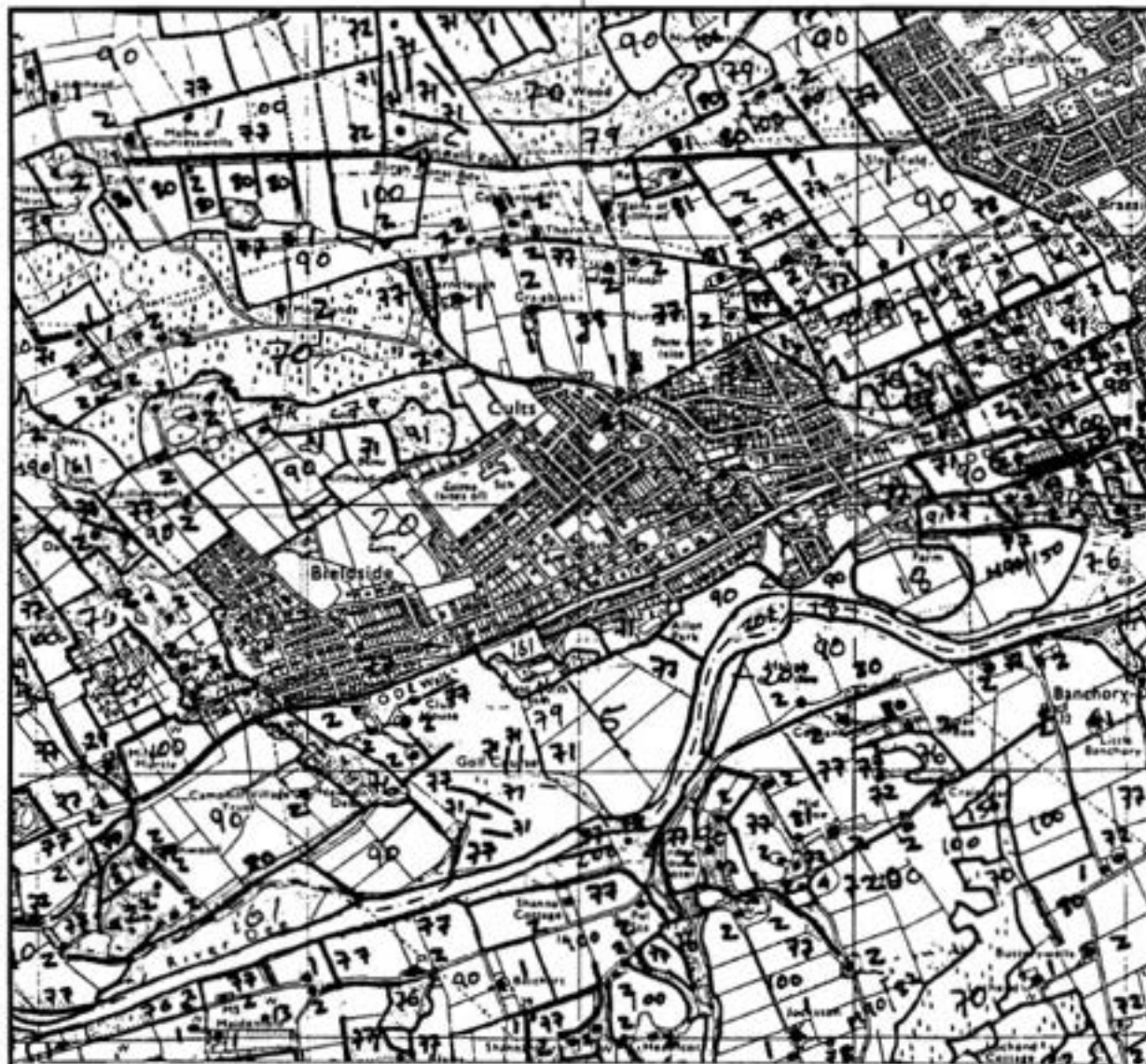
Figure 4.3 Example of base map with superimposed land cover information; area shown is to the west of Aberdeen
