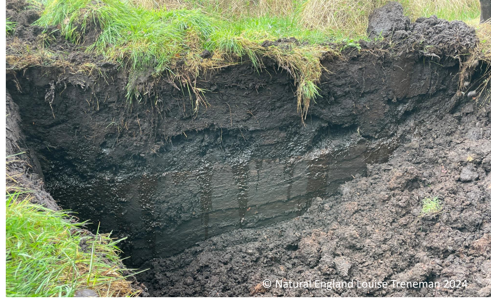
Right: subsurface seepage line – why we need deep trench bunds!
