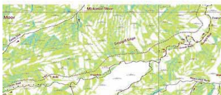
Figure 30. Topographic index calculated for blanket mire at Mickleton Moor in the northern Pennines.
